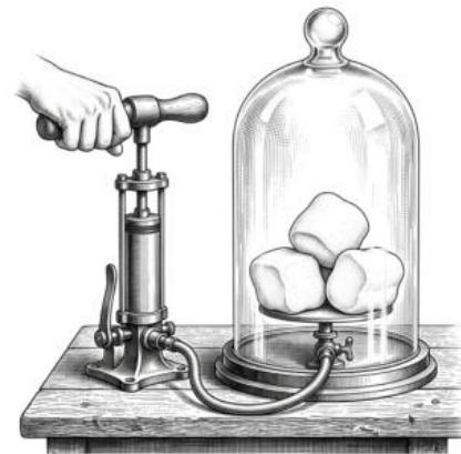
Fig. 6 — the air inside them pushes out when the jar stops pushing in
